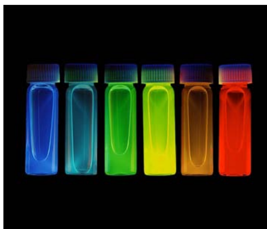
Figure 2.2 CdSe/ZnS QDs solutions under UV lamp irradiation emitting different colors, from the blue to the red, depending on their size (from 2 to 6 nm). 21
